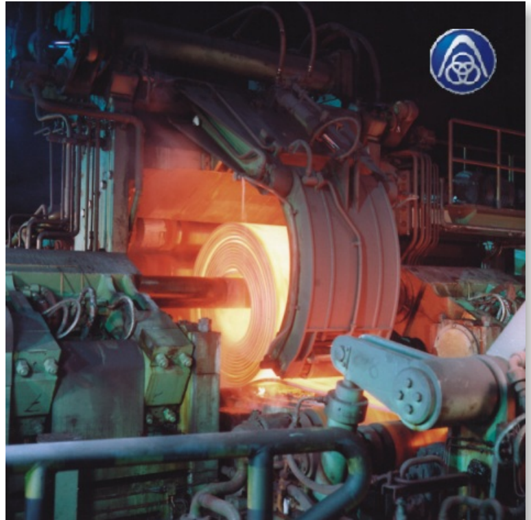
Hot rolled strip in the coiling box at TKS Bochum
